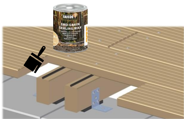
Figure 4: End-sealing with Kebony End-Grain Sealing Wax is recommended as part of best practice – this reduces the risk of ends splitting.
